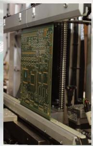
automation does not necessarily mean "High Volume", BUT the ability to test dozens of unique batches or "part numbers" of PCBs in small quantities OR large quantities.
